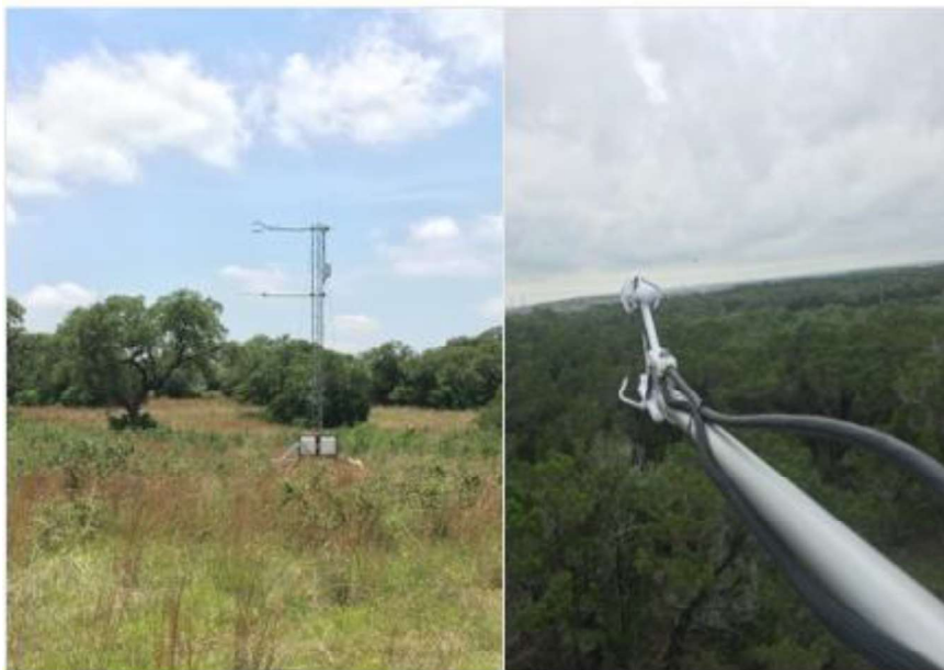
Figure 1. Images of eddy covariance towers installed at Camp Bullis site.
