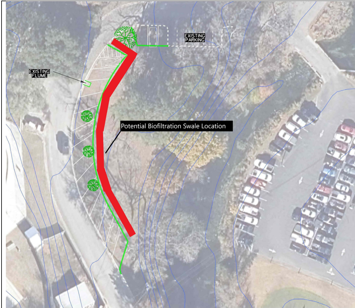
Figure 7 Golf Course Rd. Parking and Biofiltration
